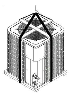
Use field-supplied spreader bars when lifting the unit to minimize the possibility of lifting cable/straps damage. To protect the cabinet louvers, use protective material such as plywood behind the cable/straps. Arrange the straps to form a central suspension point. **NOTE:** When raising and setting the unit, observe all safety rules. Remove shipping skid and all protection and lifting material after the unit is in place.
